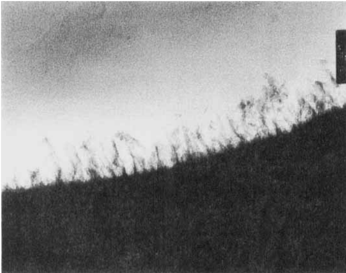
FIGURE 2 Ti-oxide layer with the Ti-surface and primer. Magnification 175,000 \times .
